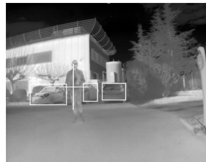
Embedded CNN inference (YoloV3)
