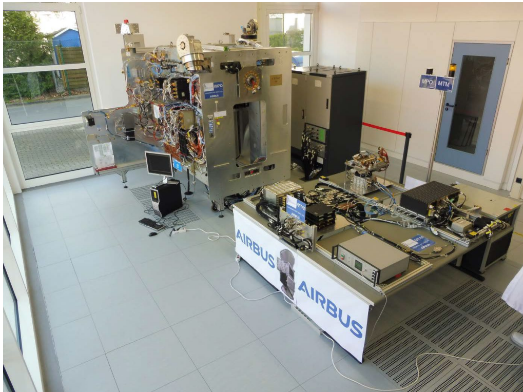
Fig. 4. BepiColombo Engineering Test Bench at ESOC
