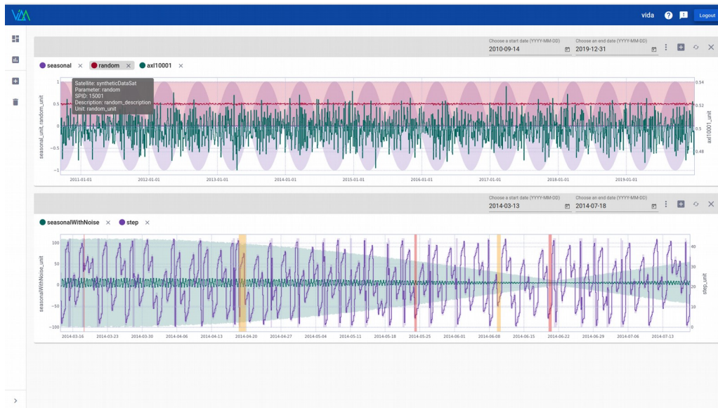
Fig. 4 Example screenshot of a Workspace with two multi-parameter plots, one of them also highlighting time periods where novelties were detected, as yellow (TD) and red (HP) vertical bars.
