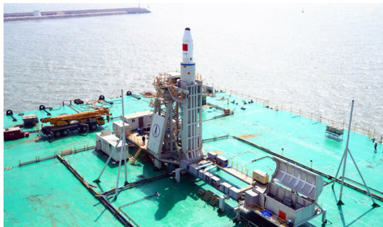
Fig. 9. LM11 erected into its silo onto the Tairui launch barge [19]
