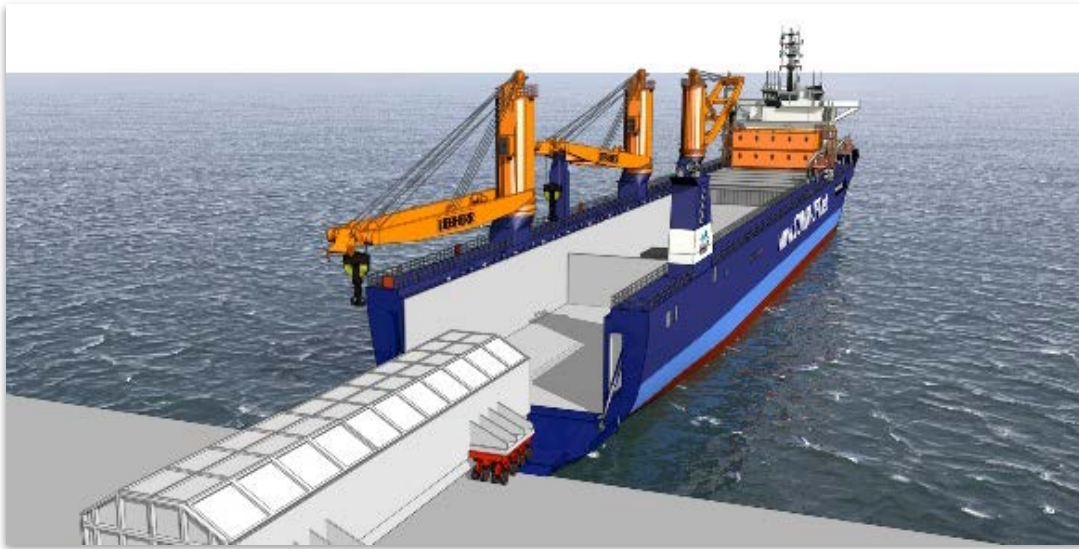
Fig. 19. Loading/Offloading of the Mobile Launch Box in Roll-in-Roll-Out Procedure
