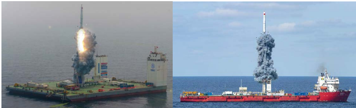
Fig. 11. LM11 launch from silo launch system from non-propelled (left, [21]) and self-propelled (right, [22]) barges
