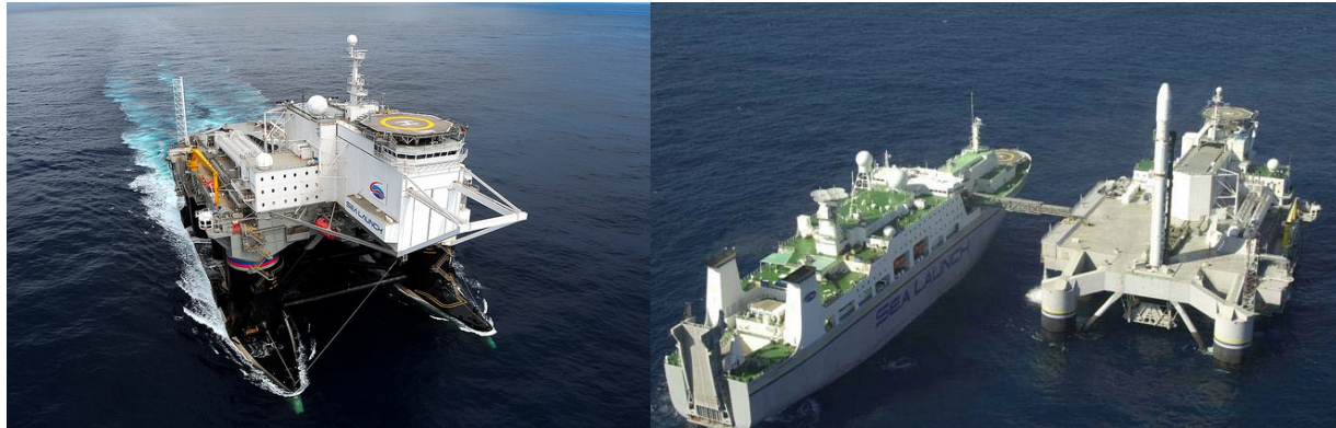
Fig. 4. The Sea Launch Platform (left, [15]) and Assembly and Command ship & Launch Platform in launch preparation configuration (right, [16])
