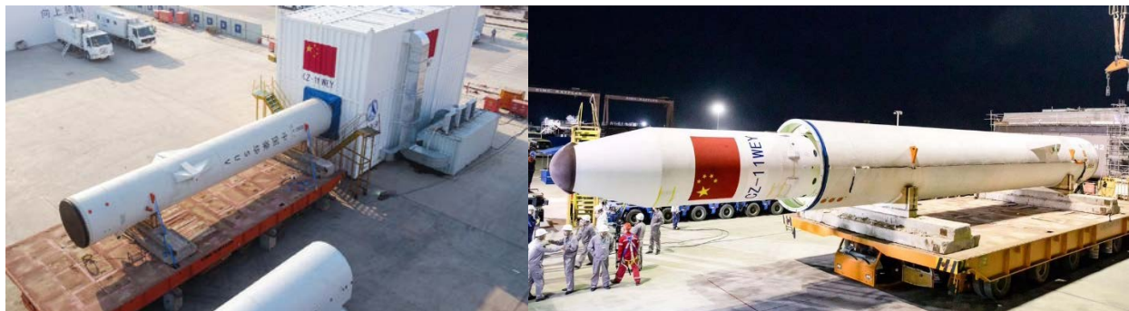
Fig. 8. LM11 launcher into its launch silo mated to the container-based fairing/payload processing facility set at homebase harbour (left,), and set onto its transporter for transfer onto launch barge (right)
