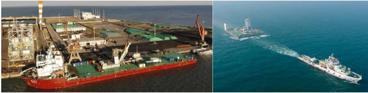
Fig. 10. LM11 erected in its silo aboard the Debo-3 self-propelled launch barge (left, [20]) and the non-propelled Tairui launch platform pulled to the launch point by a tug boat (right)
