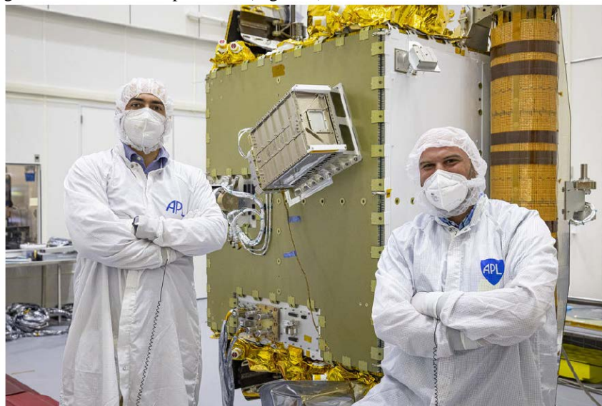
Figure 2 – LICIACube integrated on DART spacecraft
