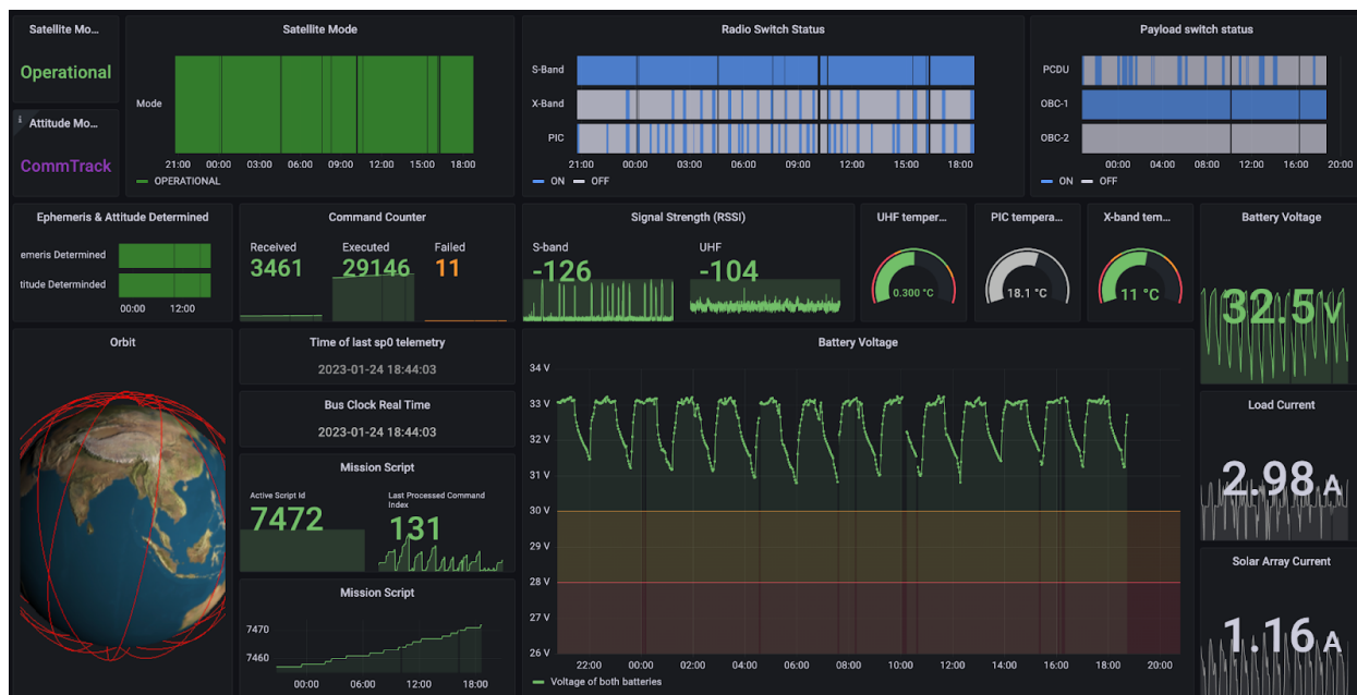
Figure 2: One of the Grafana dashboards of Cockpit, displaying a subset of spacecraft telemetry.
