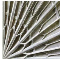
An arch is a great example: weight pressed onto the top of the arch gets distributed throughout the whole shape because it resolves forces into compressive stresses while eliminating tensile stresses. Instead, the compression dominant structural shape of the prototypes allowed for a simple interface design using only male-female interlocking features to guarantee alignment," the paper states.
